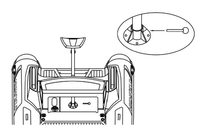
2 Insert the pin into the installation hole to lock and fix the rear tow post.
