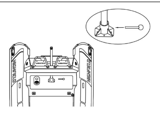
2 Insert the pin into the installation hole to lock and fix the rear tow post.
