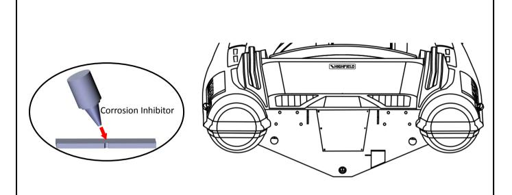
① Use insulating compound to eliminate corrosion between the aluminum and the stainless steel screws.
