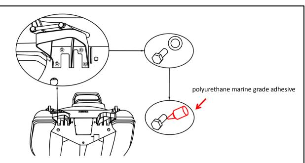
3 Secure the platform using polyurethane marine grade adhesive such as 3M 5200, Sika 291, Fixtech Fix 15.
