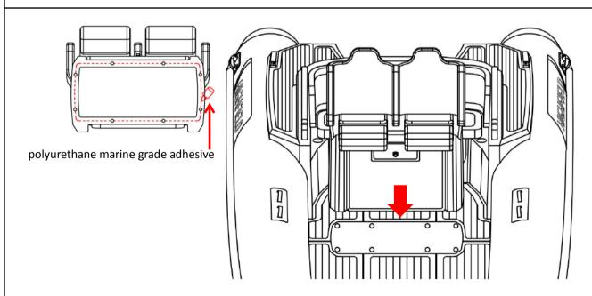
② Gently clean the deck. Secure the seat using polyurethane marine grade adhesive such as 3M 5200, Sika 291, Fixtech Fix 15.
