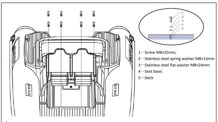
③ Use insulating compound on the M8 stainless steel screws supplied with the seat. Fasten the seat to the deck using the screws.
