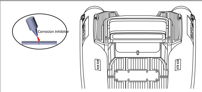
① Use insulating compound to eliminate corrosion between the aluminum and the stainless steel screws.
