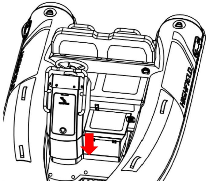
② Gently clean the deck. Secure the console using polyurethane marine grade adhesive such as 3M 5200, Sika 291, Fixtech Fix 15.
