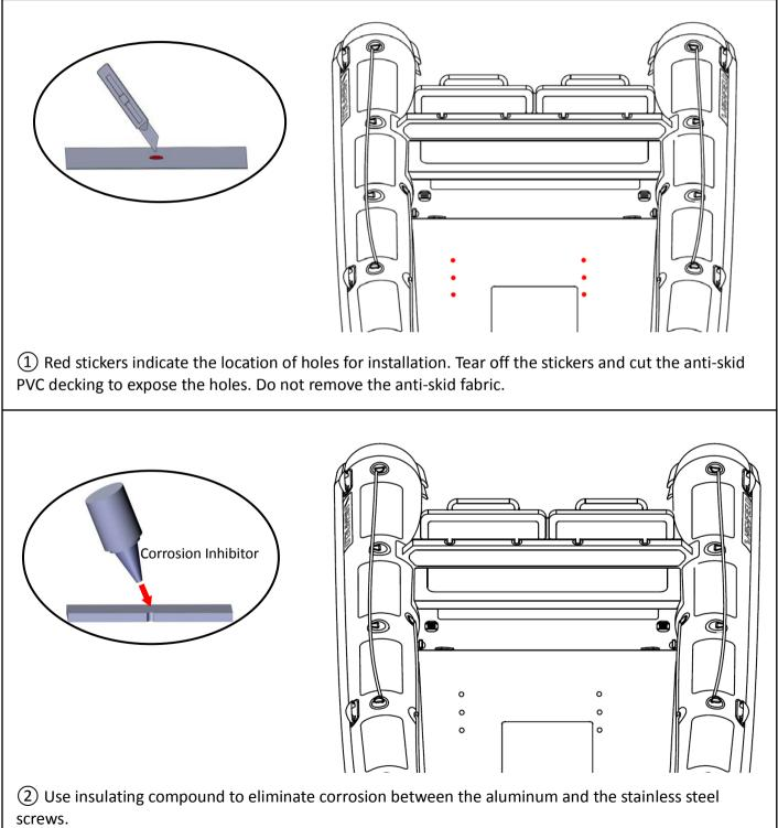
Recommended corrosion inhibitor: Duralac, Tef-Gel, Lanocote
